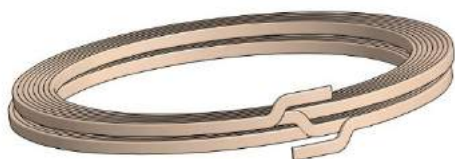
Figure 4. A pair of galleys of interleaved disk winding
